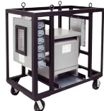
3-PHASE TRANSFORMER POWER STATION, 4 WHEELS, 480V 3P4W TO 120/208V 45PW, 15KVA TRANSFORMER Part# 6220PDC75
